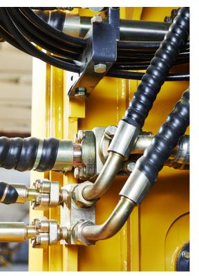
O-rings are more than just a rubber seal, there are many different types of material for many types of applications. There are also many considerations when selecting material, most importantly the combinations of fitting material and the media being transferred. Most are made of elastomers, yet there are some metal O-rings as well. Material selection is based on chemical compatibility, application temperature, sealing pressure, durometer and size.
