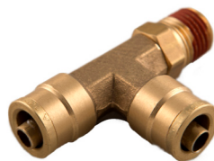
APTC71S Male Swivel Run Tee D.O.T. Push To Connect Fitting For Nylon Tube
