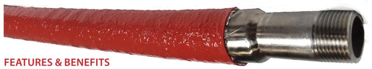
RHINO FIRESLEEVE is designed to protect hoses, wire and cables from the hazards of high heat and occasional flame. Rated for 500°F (260°C) continuous exposure, up to 2000°F (1093°C) for 15-20 minutes and up to 3000°F (1650°C) for 15-30 seconds. Made of knitted construction fiberglass yarns in a flexible substrate, it is then coated with a high-grade silicone rubber.
