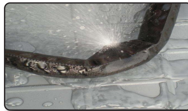
Actual picture of pin hole burst dispersion pattern at 4,000 P.S.I.
