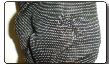
Close up of RHINO SLEEVE® HT sleeving after pin hole burst
